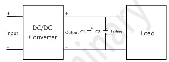
Note: The bandwidth for ripple testing is 20MHz
